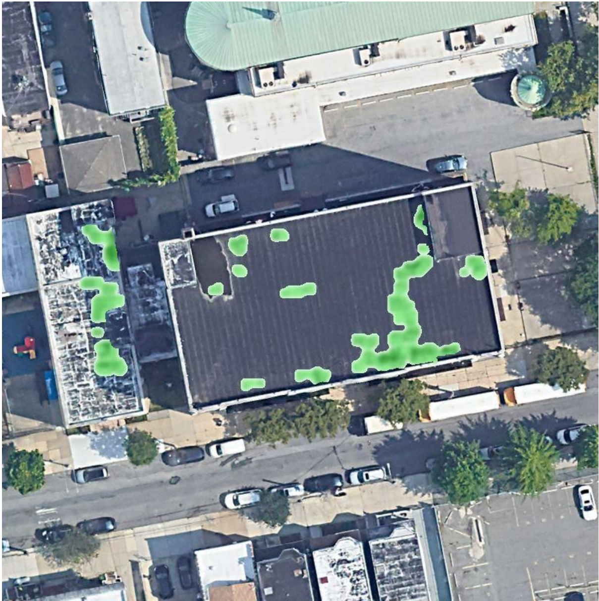
Figure 4.6: Below Membrane Moisture Map
