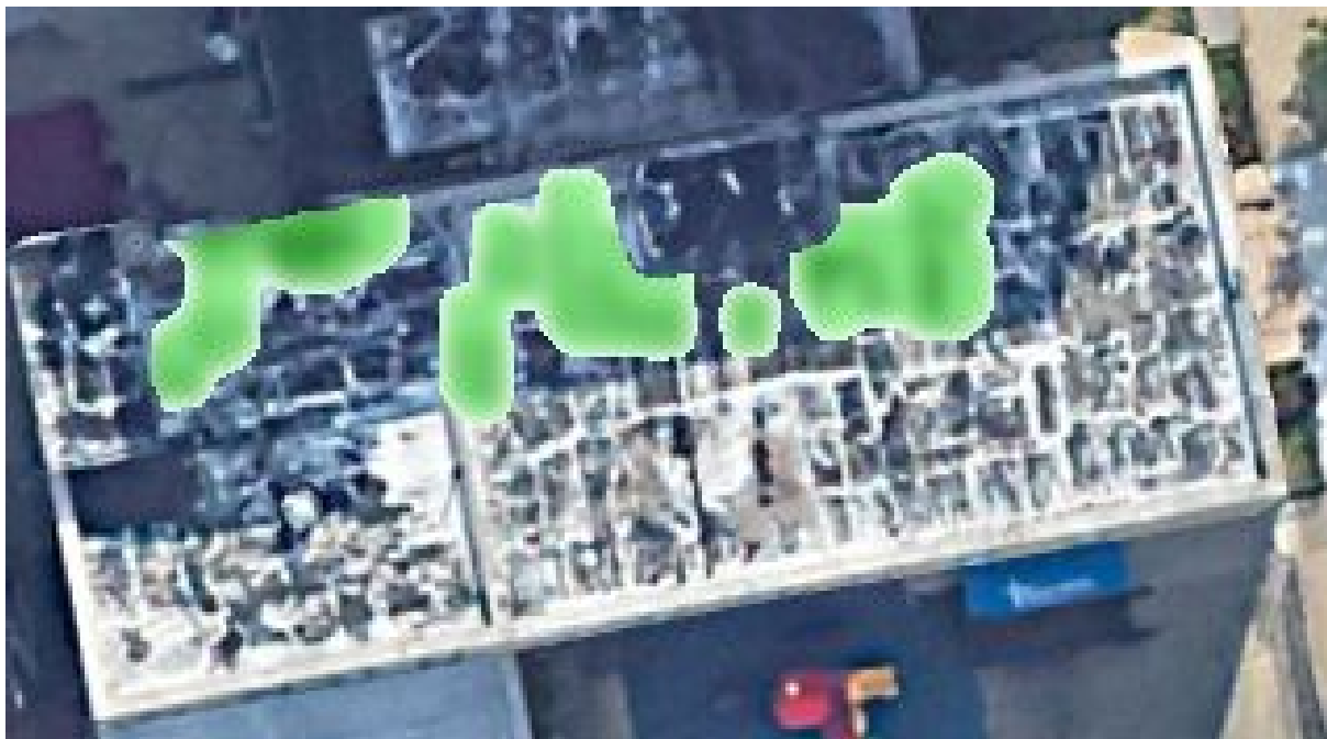
Figure 4.8: Below Membrane Moisture
