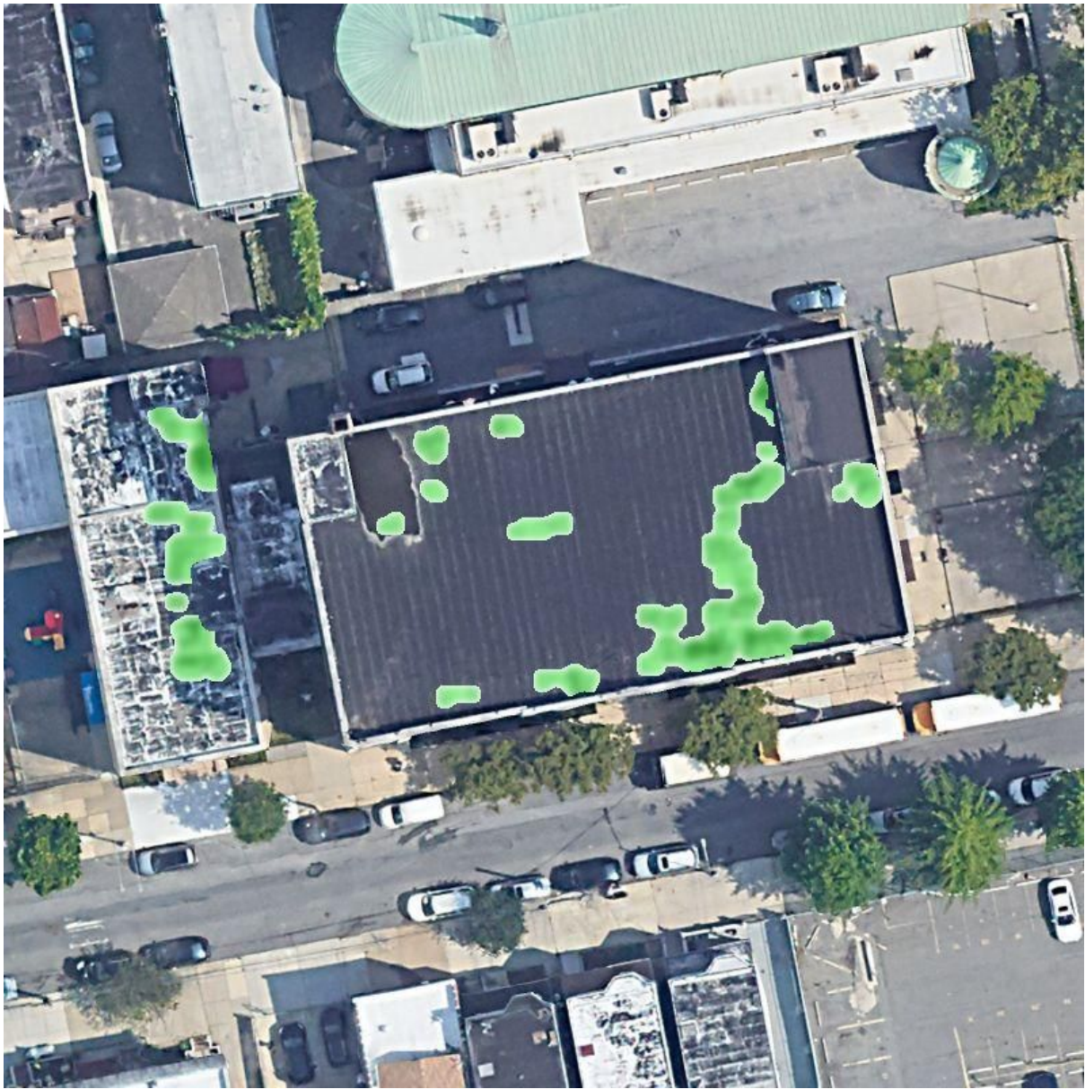
Figure 3.5: Areas in green show all detected sub-surface moisture
