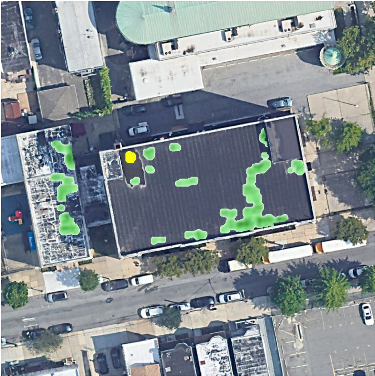
Figure 3.6: Areas in green show all detected sub-surface moisture, areas in yellow show all above-surface moisture
